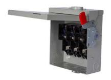
Siemens Low Voltage Circuit Protection General Duty Safety Switches. Type: ENCLOSED, SAFETY SWITCH Std: CSA V. Rating: 240V A. Rating: 60A Wattage: 3W No. Of Poles: 2P F. Rating: 60Hz Action: SINGLE THROW Material: STEEL Enclosure: TYPE 1. 2-3 point mounting holes. O. Cycles: 10000 O. Temperature: (-20F-120F) AMBIENT TEMPERATURE Environmental Conditions: INDOOR
