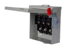
Siemens Low Voltage Circuit Protection General Duty Safety Switches. Type: ENCLOSED, SAFETY SWITCH Std: CSA V. Rating: 600V A. Rating: 100A Wattage: 3W No. Of Poles: 3P F. Rating: 60Hz Action: SINGLE THROW Material: STEEL Enclosure: TYPE 1. 2-3 point mounting holes. O. Cycles: 10000 O. Temperature: (-20F-120F) AMBIENT TEMPERATURE Environmental Conditions: INDOOR
