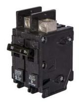
Siemens Low Voltage Molded Case Circuit Breakers General Purpose MCCBs are Circuit Protection Molded Case Circuit Breakers. 2-Pole Common-Trip circuit breaker type HBQ. Rated 120/240V (025A) (AIR 65 kA). Special features: ring tounge. Note: load side lugs are included.
