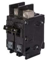
Siemens Low Voltage Molded Case Circuit Breakers General Purpose MCCBs are Circuit Protection Molded Case Circuit Breakers. 2-Pole Common-Trip circuit breaker type HBQ. Rated 120/240V (070A) (AIR 65 kA). Special features: ring tounge. Note: load side lugs are included.
