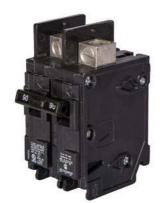
Siemens Low Voltage Molded Case Circuit Breakers General Purpose MCCBs are Circuit Protection Molded Case Circuit Breakers. 2-Pole Common-Trip circuit breaker type HBQ. Rated 120/240V (080A) (AIR 65 kA). Special features: ring tounge. Note: load side lugs are included.
