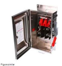
Siemens Low Voltage Circuit Protection Heavy Duty Safety Switches. Type: ENCLOSED, SAFETY SWITCH Std: UL V. Rating: 240V A. Rating: 60A Wattage: 2W No. Of Poles: 2P F. Rating: 60Hz Action: SINGLE THROW Material: SS Enclosure: TYPE 4X. 2-3 point mounting holes. Insulation: YES O. Cycles: 10000 O. Temperature: (-20F-120F) AMBIENT TEMPERATURE Environmental Conditions: INDUSTRIAL CORROSIVE RESISTANCE
