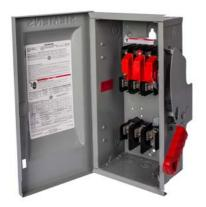
Siemens Low Voltage Circuit Protection Heavy Duty Safety Switch. 2-Pole 2-Fuse and solid neutral Fused in a type 1 enclosure (indoor). Rated 240VAC (100A).
