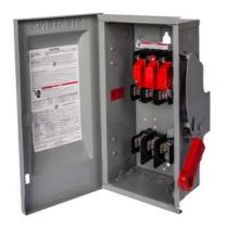
Siemens Low Voltage Circuit Protection Heavy Duty Safety Switches. Type: ENCLOSED, SAFETY SWITCH Std: UL V. Rating: 240V A. Rating: 100A Wattage: 3W No. Of Poles: 2P F. Rating: 60Hz Action: SINGLE THROW Material: 304SS Enclosure: TYPE 3R. 2-3 point mounting holes. O. Cycles: 10000 O. Temperature: (-20F-120F) AMBIENT TEMPERATURE Environmental Conditions: OUTDOOR
