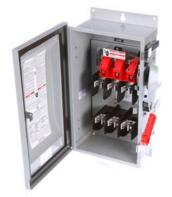
Siemens Low Voltage Circuit Protection Heavy Duty Safety Switches. Type: ENCLOSED, SAFETY SWITCH Std: UL V. Rating: 240V A. Rating: 30 A Wattage: 3W No. Of Poles: 3P F. Rating: 60Hz Action: SINGLE THROW Material: 304SS Enclosure: TYPE 12. 2-3 point mounting holes. Insulation: YES O. Cycles: 10000 O. Temperature: (-20F-120F) AMBIENT TEMPERATURE Environmental Conditions: INDUSTRIAL
