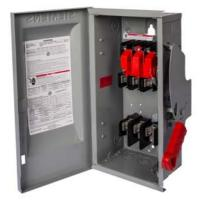
Siemens Low Voltage Circuit Protection Heavy Duty Safety Switches. Type: ENCLOSED, SAFETY SWITCH Std: UL V. Rating: 240V A. Rating: 60A No. Of Poles: 3P F. Rating: 60Hz Action: SINGLE THROW Material: SS Enclosure: TYPE 4X. 2-3 point mounting holes. Insulation: YES O. Cycles: 10000 O. Temperature: (-20F-120F) AMBIENT TEMPERATURE Environmental Conditions: INDUSTRIAL CORROSIVE RESISTANCE
