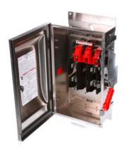
Siemens Low Voltage Circuit Protection Heavy Duty Safety Switches. Type: ENCLOSED, SAFETY SWITCH Std: UL V. Rating: 240V A. Rating: 100A Wattage: 3W No. Of Poles: 3P F. Rating: 60Hz Action: SINGLE THROW Material: SS Enclosure: TYPE 4X. 2-3 point mounting holes. Insulation: YES O. Cycles: 10000 O. Temperature: (-20F-120F) AMBIENT TEMPERATURE Environmental Conditions: INDUSTRIAL CORROSIVE RESISTANCE
