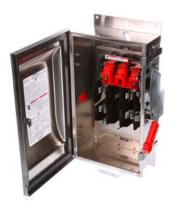
Siemens Low Voltage Circuit Protection Heavy Duty Safety Switches. Type: ENCLOSED, SAFETY SWITCH Std: UL V. Rating: 600V A. Rating: 30 A No. Of Poles: 3P F. Rating: 60Hz Action: SINGLE THROW Material: 316SS Enclosure: TYPE 4X. 2-3 point mounting holes. Insulation: YES O. Cycles: 10000 O. Temperature: (-20F-120F) AMBIENT TEMPERATURE Environmental Conditions: INDUSTRIAL CORROSIVE RESISTANCE
