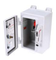
Siemens Low Voltage Circuit Protection Heavy Duty Safety Switches. Type: ENCLOSED, SAFETY SWITCH Std: UL V. Rating: 600V A. Rating: 60A Wattage: 4W No. Of Poles: 3P F. Rating: 60Hz Action: SINGLE THROW Material: NM Enclosure: TYPE 4X. 2-3 point mounting holes. Insulation: YES O. Cycles: 10000 O. Temperature: (-20F-120F) AMBIENT TEMPERATURE Environmental Conditions: INDUSTRIAL CORROSIVE RESISTANCE
