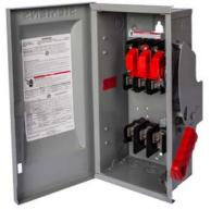
Siemens Low Voltage Circuit Protection Heavy Duty Safety Switches. Type: ENCLOSED, SAFETY SWITCH Std: UL V. Rating: 600V A. Rating: 100A No. Of Poles: 3P F. Rating: 60Hz Action: SINGLE THROW Material: 304SS Enclosure: TYPE 12. 2-3 point mounting holes. Insulation: YES O. Cycles: 10000 O. Temperature: (-20F-120F) AMBIENT TEMPERATURE Environmental Conditions: INDUSTRIAL
