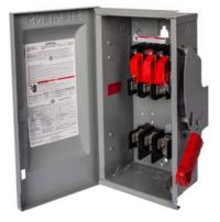
Siemens Low Voltage Circuit Protection Heavy Duty Safety Switches. Type: ENCLOSED, SAFETY SWITCH Std: UL V. Rating: 600V A. Rating: 100A Wattage: 4W No. Of Poles: 3P F. Rating: 60Hz Action: SINGLE THROW Material: STEEL Enclosure: TYPE 1. 2-3 point mounting holes. O. Cycles: 10000 O. Temperature: (-20F-120F) AMBIENT TEMPERATURE Environmental Conditions: INDOOR
