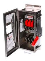
Siemens Low Voltage Circuit Protection Heavy Duty Safety Switches. Type: ENCLOSED, SAFETY SWITCH Std: UL V. Rating: 600V A. Rating: 100A No. Of Poles: 3P F. Rating: 60Hz Action: SINGLE THROW Material: SS Enclosure: TYPE 4X. 2-3 point mounting holes. Insulation: YES O. Cycles: 10000 O. Temperature: (-20F-120F) AMBIENT TEMPERATURE Environmental Conditions: INDUSTRIAL CORROSIVE RESISTANCE
