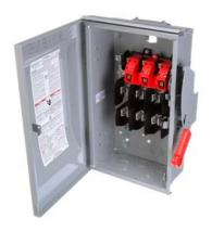
Siemens Low Voltage Circuit Protection Heavy Duty Safety Switches. Type: ENCLOSED, SAFETY SWITCH Std: CSA V. Rating: 240V A. Rating: 30 A Wattage: 4W No. Of Poles: 3P F. Rating: 60Hz Action: SINGLE THROW Material: 304SS Enclosure: TYPE 3R. 2-3 point mounting holes. O. Cycles: 10000 O. Temperature: (-20F-120F) AMBIENT TEMPERATURE Environmental Conditions: OUTDOOR
