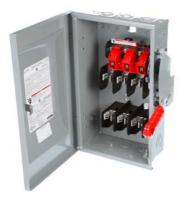
Siemens Low Voltage Circuit Protection Heavy Duty Safety Switches. Type: ENCLOSED, SAFETY SWITCH Std: CSA V. Rating: 600V A. Rating: 60A Wattage: 4W No. Of Poles: 3P F. Rating: 60Hz Action: SINGLE THROW Material: 304SS Enclosure: TYPE 3R. 2-3 point mounting holes. O. Cycles: 10000 O. Temperature: (-20F-120F) AMBIENT TEMPERATURE Environmental Conditions: OUTDOOR
