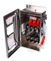
Siemens Low Voltage Circuit Protection Heavy Duty Safety Switches. Type: ENCLOSED, SAFETY SWITCH Std: CSA V. Rating: 600V A. Rating: 60A Wattage: 3W No. Of Poles: 3P F. Rating: 60Hz Action: SINGLE THROW Material: SS Enclosure: TYPE 4X. 2-3 point mounting holes. Insulation: YES O. Cycles: 10000 O. Temperature: (-20F-120F) AMBIENT TEMPERATURE Environmental Conditions: INDUSTRIAL CORROSIVE RESISTANCE
