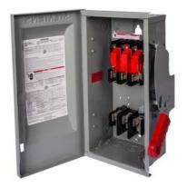
Siemens Low Voltage Circuit Protection Heavy Duty Safety Switches. Type: ENCLOSED, SAFETY SWITCH Std: CSA V. Rating: 600V A. Rating: 200A Wattage: 4W No. Of Poles: 3P F. Rating: 60Hz Action: SINGLE THROW Material: 304SS Enclosure: TYPE 3R. 2-3 point mounting holes. O. Cycles: 8000 O. Temperature: (-20F-120F) AMBIENT TEMPERATURE Environmental Conditions: OUTDOOR
