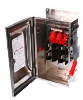
Siemens Low Voltage Circuit Protection Heavy Duty Safety Switches. CSA 200A 3P 3W 600V FUSED HD TY 4X
