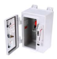
Siemens Low Voltage Circuit Protection Heavy Duty Safety Switches. Type: ENCLOSED, SAFETY SWITCH Std: UL V. Rating: 600V A. Rating: 30 A Wattage: 3W No. Of Poles: 3P F. Rating: 60Hz Action: SINGLE THROW Material: NM Enclosure: TYPE 4X. 2-3 point mounting holes. Insulation: YES O. Cycles: 10000 O. Temperature: (-20F-120F) AMBIENT TEMPERATURE Environmental Conditions: INDUSTRIAL CORROSIVE RESISTANCE
