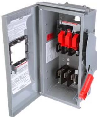
Siemens Low Voltage Circuit Protection Heavy Duty Safety Switch. 3-Pole Non-Fused in a type 3R enclosure (outdoor). Rated 600VAC (60A). Special features: viewing window.
