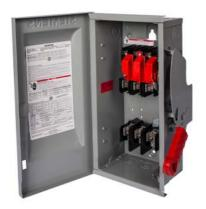
Siemens Low Voltage Circuit Protection Heavy Duty Safety Switch. 3-Pole 3-Wire Non-Fused in a type 3R enclosure (outdoor). Rated 600VAC (100A). Special features: photovoltaic rated, positive ground, 10000 AIC disconnect
