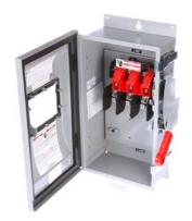
Siemens Low Voltage Circuit Protection Heavy Duty Safety Switches. CSA 60A 3P 600V 3W NON-FUSED HD TYPE 12  $\,$
