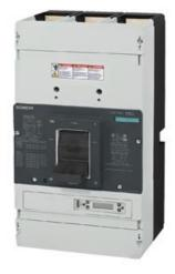
CIRCUIT-BREAKER VL 1200 UL; TYPE NG (CAT NO. HNX3B120) NON-INTERCHANGEABLE FRAME W. APPROBATION CIRCUIT-BREAKER TO UL489 HIGH BREAKING CAPACITY 3-POLE, NEMA RATING 65KA/480V, (MOLDED CASE CIRCUIT BREAKER) OVERCURRENT RELEASE TM, LI TU= 40 DEGR. CELSIUS IN= < 1200A, RATED CURRENT II= 7000...12000A SHORT-CIRCUIT PROTECTION IR= 1200A OVERCURRENT RELEASE F. PLANT PROTECTION W/O CONNECTION ACCESSORIES WITHOUT AUXILIARY RELEASE WITHOUT AUXILIARY/ALARM SWITCH
