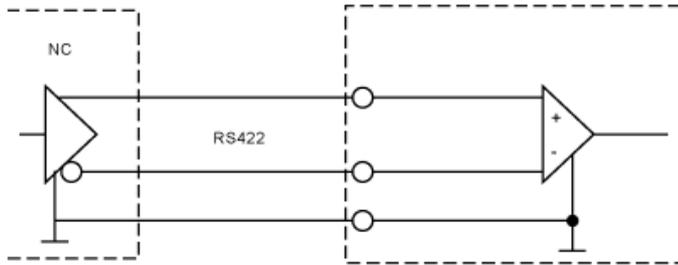
The reference pulses are supplied via two of the signal inputs, either as pulse/ direction signals or as A/B signals. The other signal inputs have the functions "power amplifier enable/pulse blocking" and "step size switching/PWM motor current control".
