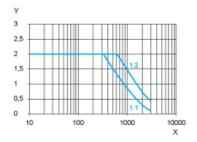
X Speed of rotation in rpm Y Torque in Nm 1.1 Max. torque at 24 V 1.2 Max. torque at 48 V
