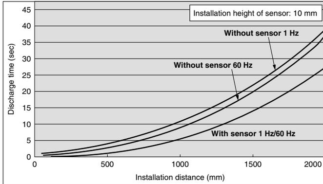
**Air purge: Yes** Supply pressure: 0.1 MPa (7  $\ell$ /min (ANR) per nozzle)
