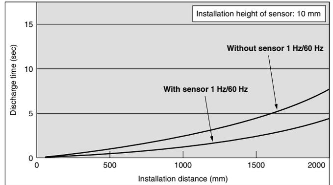
**Air purge: Yes** Supply pressure: 0.7 MPa (30  $\ell$ /min (ANR) per nozzle)
