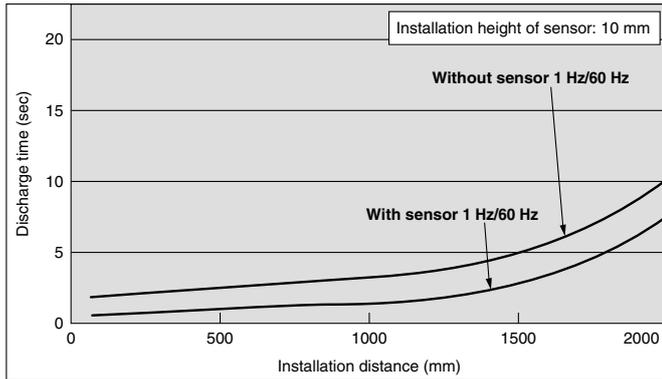
**Air purge: Yes** Supply pressure: 0.5 MPa (20  $\ell$ /min (ANR) per nozzle)
