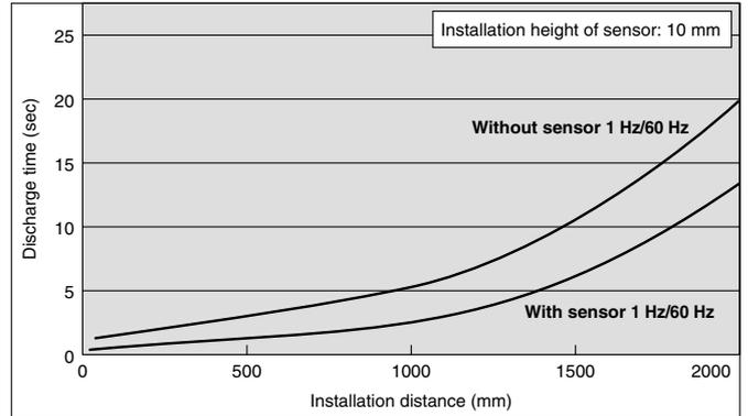
**Air purge: Yes** Supply pressure: 0.3 MPa (14  $\ell$ /min (ANR) per nozzle)
