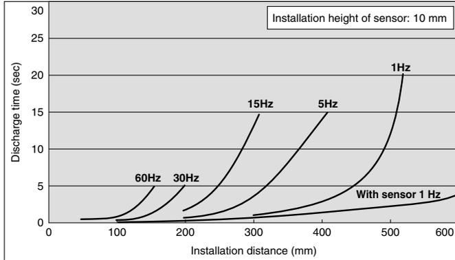
**Air purge: Yes** Supply pressure: 0.05 MPa (3.5  $\ell$ /min (ANR) per nozzle)
