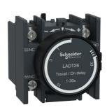
Time delay auxiliary contact block, TeSys Deca, 1NO+1NC, on delay 1-30s, front, lugs-ring terminals
