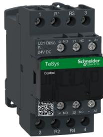
IEC contactor, TeSys Deca, nonreversing, 20A resistive, 4 pole, 2 NO and 2 NC, low consumption 24VDC coil, open style
