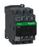
IEC contactor, TeSys Deca, nonreversing, 9A, 5HP at 480VAC, up to 100kA SCCR, 3 phase, 3 NO, 125VDC coil, open style
