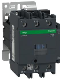
IEC contactor, TeSys Deca, nonreversing, 95A, 60HP at 480VAC, 3 phase, 3 pole, 3 NO, 24VDC coil, open style
