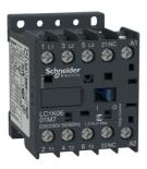
TeSys K contactor - 3P - AC-3 <= 440 V 9 A - 1 NC aux. - 220...230 V AC coil
