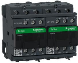
IEC contactor, TeSys Deca reversing, 12A, 7.5HP at 480VAC, 3 phase, 3 pole, 3 NO, 120VAC 50/60Hz coil, open style
