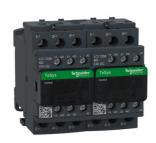
Reversing Contactor, TeSys Deca, 3P(3NO),AC-3, <=440V 38A,24V DC coil, screw clamp terminals
