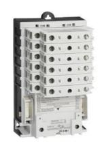
Electrically held lighting contactor, (convertible to mech. held), Amp rating 30A (tungsten 20A), 0 N.C. / 6 N.O. poles, 115-120V 60Hz/110V 50Hz coil, Non-combination type, Enclosure NEMA type (open), No enclosure
