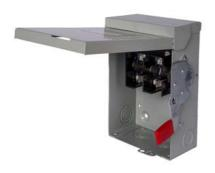
Siemens Low Voltage Circuit Protection General Duty Safety Switches. Type: ENCLOSED, SAFETY SWITCH Std: UL V. Rating: 240V A. Rating: 60A No. Of Poles: 2P F. Rating: 60Hz Action: SINGLE THROW Material: 304SS Enclosure: TYPE 3R. 2-3 point mounting holes. O. Cycles: 10000 O. Temperature: (-20F-120F) AMBIENT TEMPERATURE Environmental Conditions: OUTDOOR
