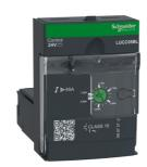
Advanced control unit, TeSys Ultra, 1.25A to 5A, 1P motors, protection & diagnostic, class 10, coil 24VDC
