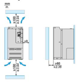
LXM32MD85N4, LXM32MC10N4 servo drives have an integrated fan.
