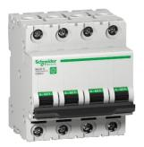
Miniature circuit breaker (MCB), Multi9 C60SP, 4P, 6A, B curve, 10kA (UL1077), 10kA (IEC/EN 60947-2)
