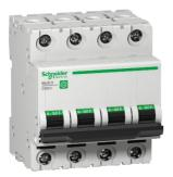
Miniature circuit breaker (MCB), Multi9 C60SP, 4P, 40A, B curve, 5kA (UL1077), 10kA (IEC/EN 60947-2)
