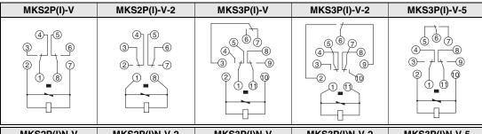
Models with LED indicator and Varistor (AC Coil)
