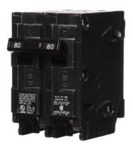
Siemens Low Voltage Residential Circuit Breakers Miniature Thermal Mag Circuit Breakers - Type QP/MP, 2-Pole, 120/240VAC are Circuit Protection Load Center Mains, Feeders, and Miniature Circuit Breakers. Type: MP-T Application: For Use In 125 AMP And 225 AMP Single Phase Output WMM, WML, WMT meter stacks Standard: HACR Rated Voltage Rating: 120/240 Amperage Rating: 80 Interrupt Rating: 10 Number Of Poles: 2 Operating Temperature: 40
