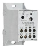
Power distribution block, Linergy, enclosed, 335A CU, 270A AL, 600V, 2 line side lug, 8 load side lug, AL lug, rail
