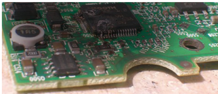
Effects of overvoltage surges on electronic equipment
