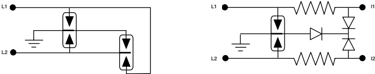
OVR TC 200 V in parallel OVR TC / xx V / 200 FR in series
