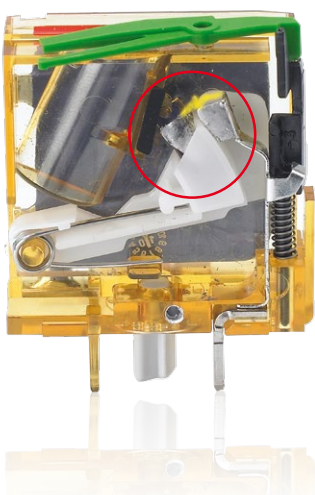
At the end of life, the opening of the thermal disconnecter and ignition of an electric arc in direct current
