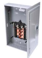
SIEMENS LOW VOLTAGE PL SERIES LOAD CENTER. MAIN LUG WITH 12 1-Inch Spaces ALLOWING MAX 24 CIRCUITS. 1-PHASE 3-WIRE SYSTEM RATED 120/240V(200A) 100KA INTERRUPT. SPECIAL FEATURES: COPPER BUS, INTERCHANGEABLE MAIN, GRAY TRIM, NEMA TYPE1 ENCLOSURE FOR INDOOR USE. REPLACED BY PN1224L1200C. AVAILABLE 4/1/2020
