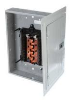
SIEMENS LOW VOLTAGE PL SERIES LOAD CENTER. MAIN LUG WITH 16 1-Inch Spaces ALLOWING MAX 24 CIRCUITS. 1-PHASE 3-WIRE SYSTEM RATED 120/240V(125A) 100KA INTERRUPT. SPECIAL FEATURES: COPPER BUS, INTERCHANGEABLE MAIN, SPLIT GROUND, GRAY TRIM, NEMA TYPE1 ENCLOSURE FOR INDOOR USE. REPLACED BY PN1632L1125C. AVAILABLE 4/1/2020
