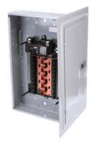
SIEMENS LOW VOLTAGE PL SERIES LOAD CENTER. FACTORY INSTALLED MAIN BREAKER WITH 20 1-INCH SPACES ALLOWING MAX 30 CIRCUITS. 1-PHASE 3-WIRE SYSTEM RATED 120/240V (150A) 22KA INTERRUPT. SPECIAL FEATURES: COPPER BUS, INTERCHANGEABLE MAIN, GRAY TRIM, NEMA TYPE1 ENCLOSURE FOR INDOOR USE. REPLACED BY PN2040B1150C. AVAILABLE 4/1/2020
