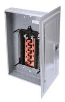
SIEMENS LOW VOLTAGE PL SERIES LOAD CENTER. MAIN LUG WITH 20 1-Inch Spaces ALLOWING MAX 30 CIRCUITS. 1-PHASE 3-WIRE SYSTEM RATED 120/240V(150A) 100KA INTERRUPT. SPECIAL FEATURES: COPPER BUS, INTERCHANGEABLE MAIN, SPLIT GROUND, GRAY TRIM, NEMA TYPE1 ENCLOSURE FOR INDOOR USE. REPLACED BY PN2040L1150C. AVAILABLE 4/1/2020
